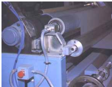
Multi-Zone Web Tension Measurement and Control
