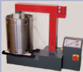
Special sliding yoke heater to heat up big e-motor housings.
