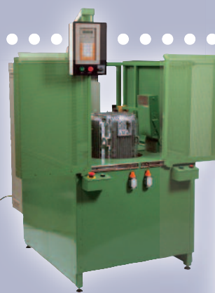
Special sliding yoke heater to heat up the tires.
