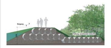
The upgrading of existing dikes can be done by using topotubes.
