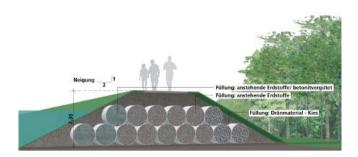
topotubes offers new construction methods for the design of dyke profiles. Through the use of geotextile tubes as a core element erosion safety is increased. By covering the outer layer with normal soil and applying a grass cover, the dyke also adds further harmony to the surrounding landscape.
