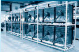
We mount several standard coolers together on a rack to increase the cooling performance (from 2 to 16 coolers).
