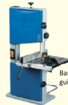
Band saws (for cutting wear and guide rings)
