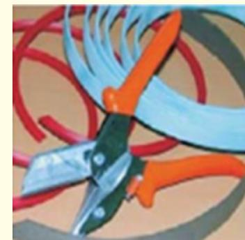
Beveling shears for cutting guide tapes
