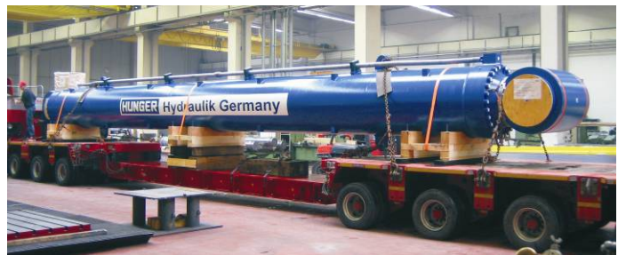
Piling Barge Cylinder – Large Cylinder with Piston Diameter of 1 m and stroke of 12.5 m
