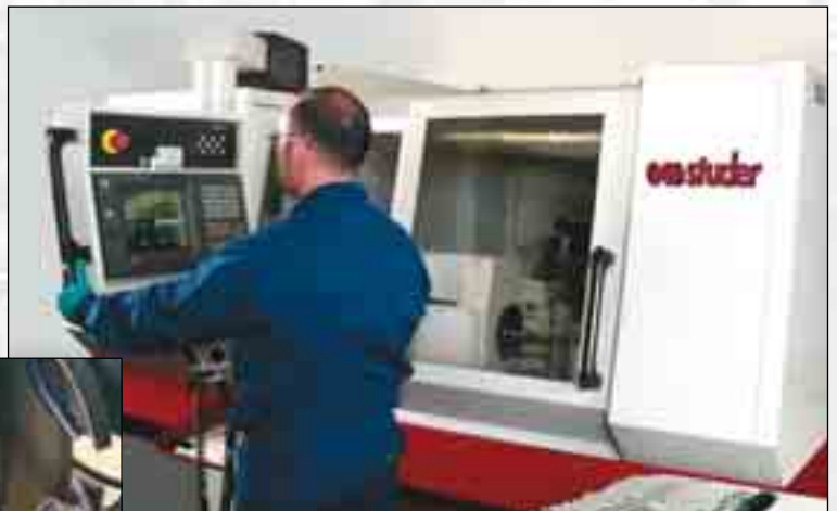
CNC - outside and inside grinding
