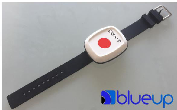
BlueBeacon SafeBand is a wearable BLE tag designed for localization and safety of workers in industrial environments.
