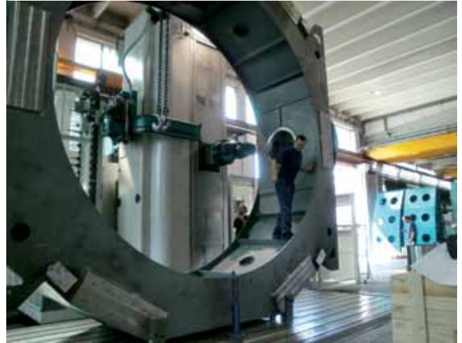
Machining of an electrowelded frame for a radar antenna
