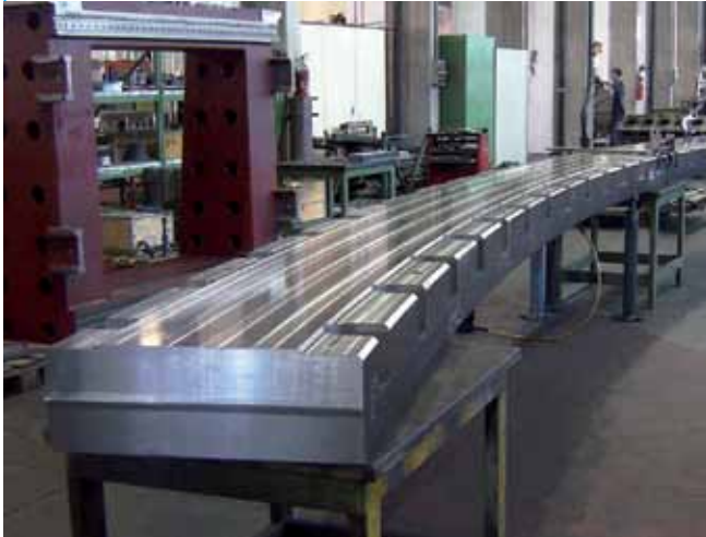
Antenna frame segments
