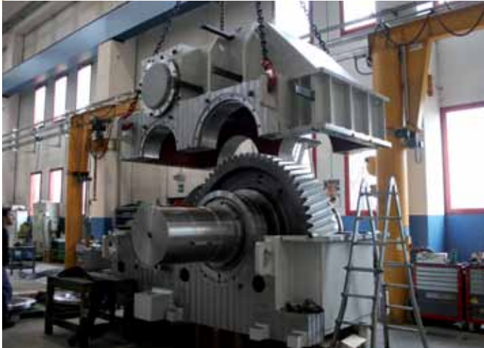
Cement Mill Drives
