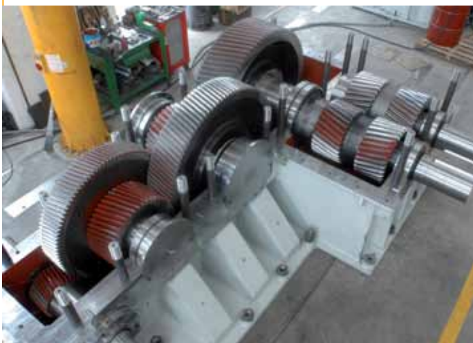
Rubber mixer drive 2500 kw at 77 rpm
