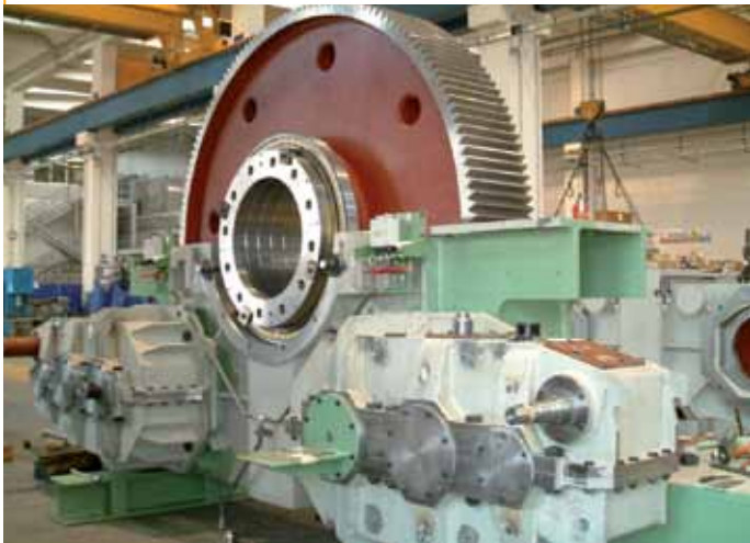
Four motor tilting converter drive unit with during assembly and intermediate geometrical inspection
