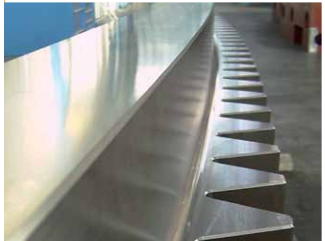
Gear toothed segments for parabolic antenna and radiotelescope application
