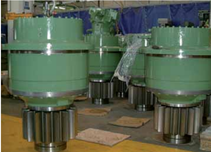
Planetary drives for "TBM" rotating head
