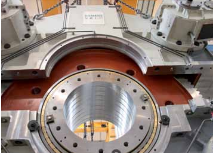
Tilting converter drives/Steel Industry (350 ton)
