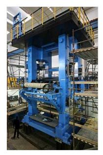
Special accessories for mill stands: AG Cylinders, Sliding Blocks, Rails, Base Plates, hydraulic strip feed and unloading systems, etc. Backup mill stand chokes, and Bending & Shifting Blocks are also manufactured and preassembled within our supply. See also: Rolling mills: roughing and finish machining of housings Rolling mills: pre-assembly, piping and inspections Sheet Mill: 4,300 mm wide - Video
