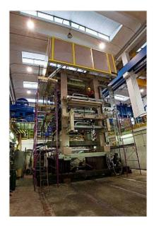
Fully assembled "Skin-Pass" stand including piping and wiring; total weight 200 ton. See also: Mills: machining and shoulder roughing Mills: pre-assembly, piping and inspections Mill Stand Chokes, AG Cylinders, and Accessories Sheet mill: 4,300 mm width – Video
