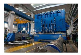
Two **hydraulic rocking shears** at the end of the pre-assembly phase in the Galbiati Group workshop. The **blade is driven** by the coordinated movement of two, approx. 1000 mm diameter, hydraulically driven pistons. Rated up to 450 bar. Total weight: more than 450 ton each. **See also: Mechanical Rocking Shear Mechanical Rocking Shear – Video Pendular shear for thin sheets Gear Trains for Mechanical Rocking Shear**
