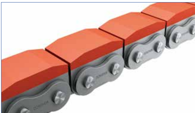
Conveyor chain for sensitive goods with elastomer of NBR or PU available in different shore hardnesses
