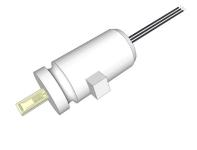
The standard FS5.A measures  $\emptyset$  6.0 (±0.1) mm, L = 14 (±0.2) mm. PTFE wires measure 195 mm.
