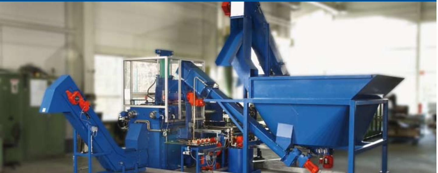
Hydraulic briquetting press with corresponding materials handling technology
