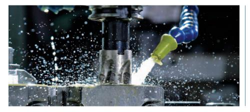
A thorough cleaning extends the lifespan of cooling lubricants and improves the surface quality that can be achieved during processing.
