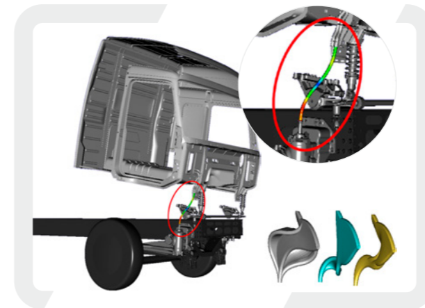
Stress on supplying hose of a driver's cabin while tilting and envelopes of needed installation space for variations of length and fastening
