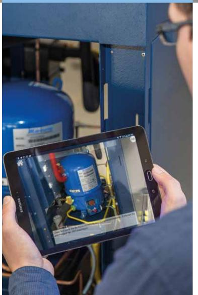
trainees can work with a virtual image of a machine. Thanks to the high degree of immersion (i.e. the realistic feel of the virtual world), the experience gained on the training object is almost as authentic as when operating the actual machine.
