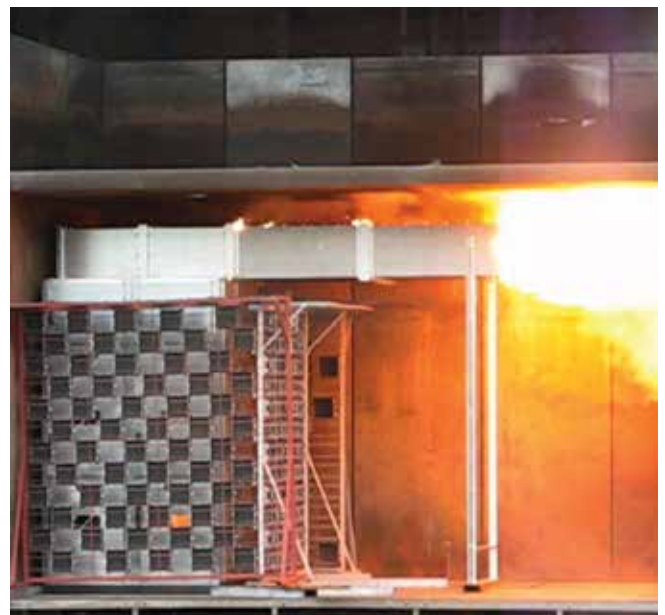
Internal arc fault test, 31.5kA/1s
