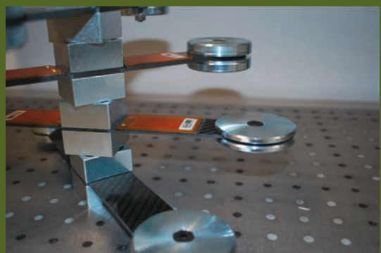
Picture 1: Active vibration decoupling with piezoceramic transducers.
