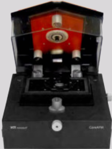
In its closed state (top), the CoreAFM's scanner compartment protects your scans from outside disturbances. It can easily be opened (bottom) to allow access to the scanner and sample stage, for example for placing a new sample.
