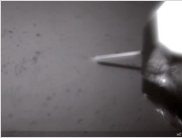
Simultaneous side view image of the same cantilever and sample. Availability of side view is ideal for a first coarse approach.
