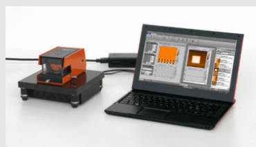
Setup. A NaioAFM, a USB cable, and a PC are all that you need!
