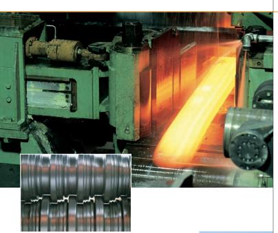
During the production of special profiles by hot rolling the input stock is shaped by two cylindrical, opposed rotating rolls into lengths up to 70 m. The products of this forming technique are employed in the most diverse economic situations. Hot rolled special profiles offer innovative solutions throughout many industries – whether it be for automotive, transport or railroad use.
