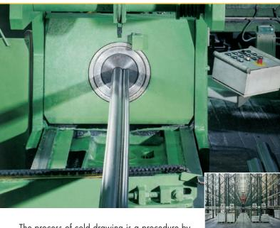
The process of cold drawing is a procedure by which the metal is formed in order to achieve complex profile cross sections of excellent precision. Special profile bars are drawn through a forming die following careful pre-treatment and descaling in one or more operations.
