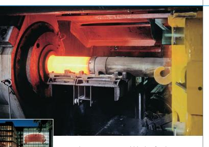
During hot extrusion a steel block, after leaving the furnace, is pressed into a profile bar (through a forming die) using a ram and an extrusion force of 2,200 t. Hot extrusion offers substantial advantages in comparison to such procedures as rolling, forging or machining.
