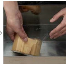
The support material can be removed easily just by soaking the model into water even for assembly parts and complex shapes.
