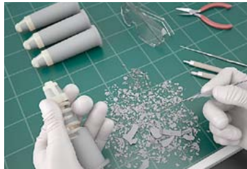
labour costs result when the removal of support material is performed manually.
