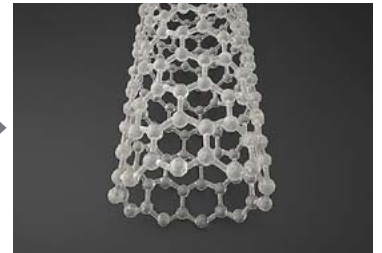
Example of the same model with the support material removed by soaking the model in water
