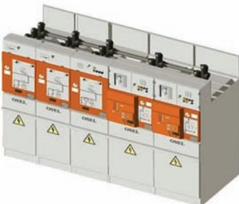
You can touch the solid insulated busbars when the system energized. All outside of the solid insulated busbars covered with semi-conductor and earthed.
