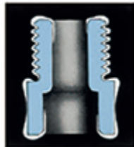
Electrolytic (galvanic) deposit
