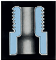
Electroless nickel deposit
