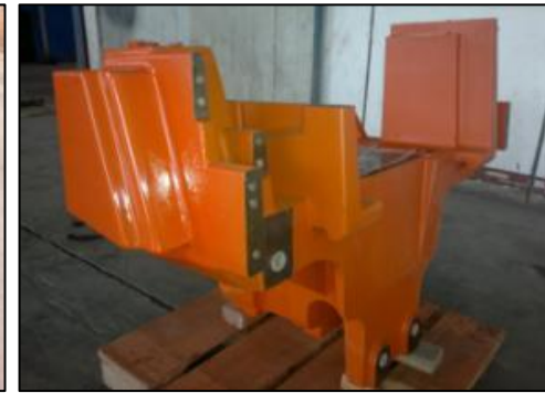
TMHMI Rear-Frame (top-coat, CNC machined)
