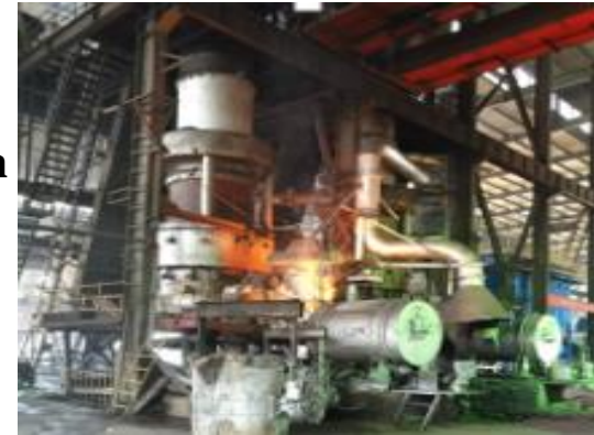
2 x medium frequency furnace/ Vacuum (up to 1ton/hr)
