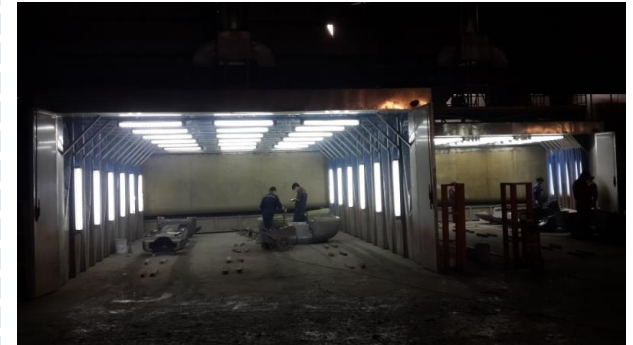
3 x Telescopic primer booth (up to 5000tons/month)
