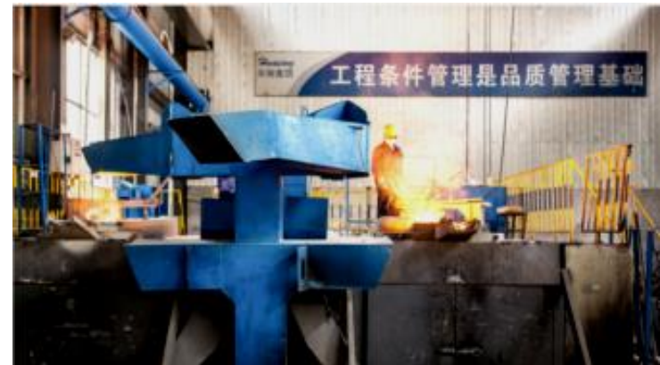
2 x medium frequency furnace/ Vacuum (up to 1ton/hr)
