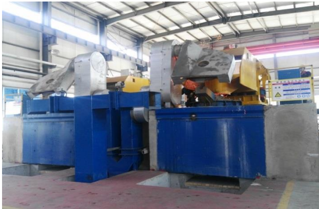
2 x medium frequency furnace/ Resin sand (up to 3tons/hr)
