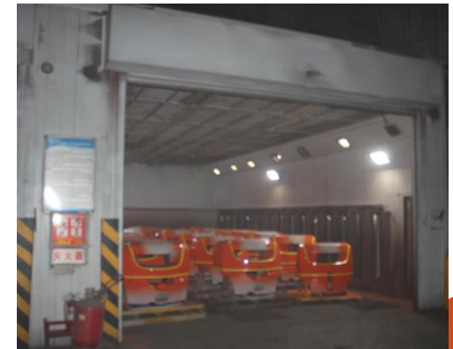
3 x Top-coat spray booths (up to 4000tons/month)
