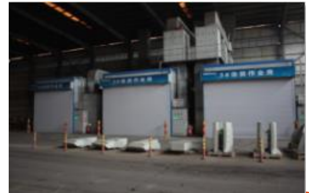
3 x primer grinding booth (up to 5000tons/month)
