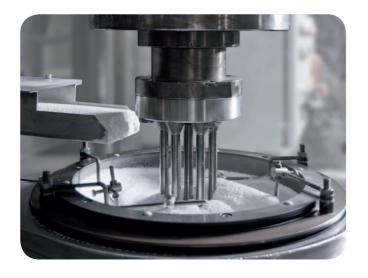
PTFE processing is very different from processing the usual thermoplastics. Injection moulding cannot be used due to the material's high melting viscosity (at very high temperatures, PTFE is merely highly viscous). The semi-finished products can therefore only be produced using Press- & Sinter- technology and RAM extrusion.
