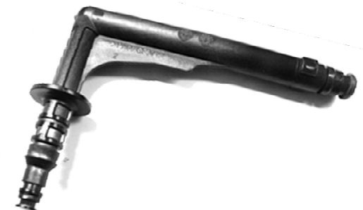
Hydraulic clutch circuit
