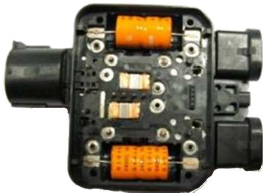
Power circuits for electronic unit to regulate radiator fan brush and brushless motor (up to 100 A)
