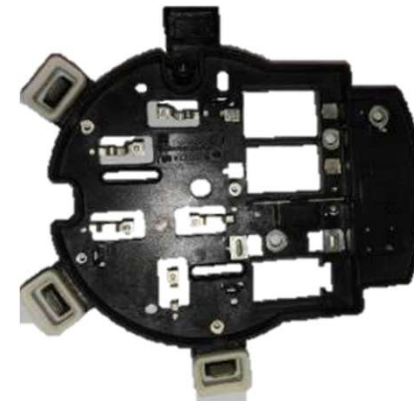
Power circuits for electronic unit to regulate radiator fan brush and brushless motor (up to 100 A)
