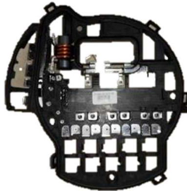
Power circuits for electronic unit to regulate radiator fan brush and brushless motor (up to 100 A)
