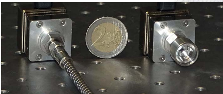
Fig. 1 Photograph of two exemplary microspectrometers, one featuring fibre coupling (left) and one featuring free-space coupling using collimation optics (right). € 2.- coin added for scale.
