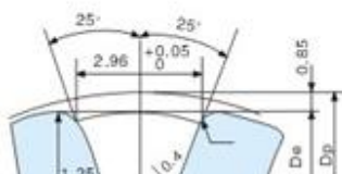
T5型齿形图: Tooth form diagram
