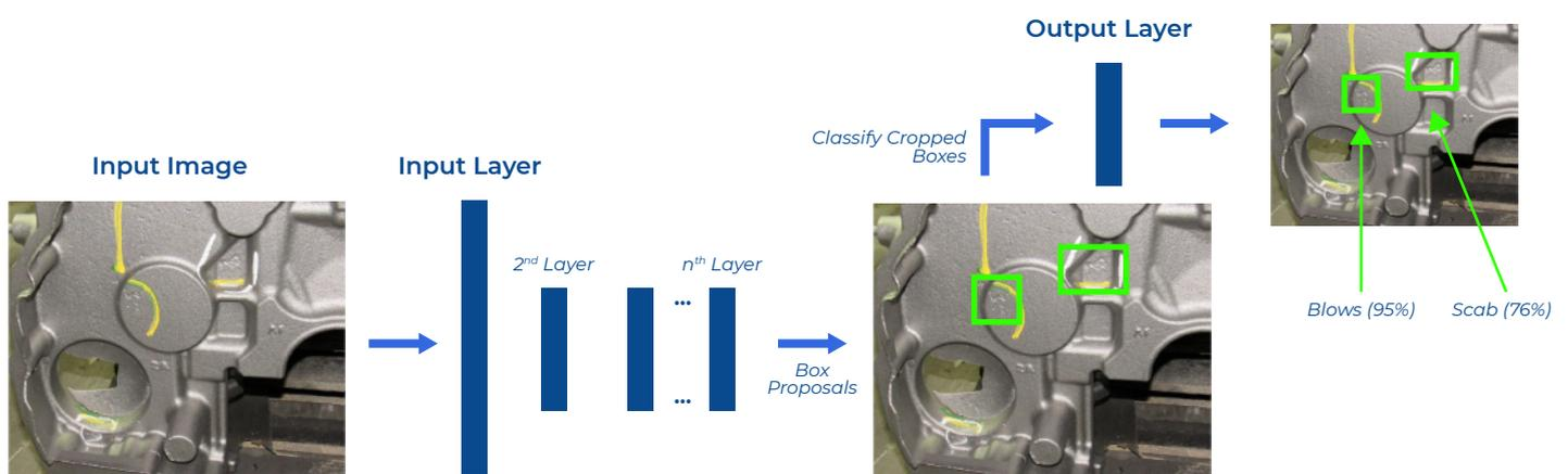
After training, DataProphet's model was applied locally upon new images. The model works by finding anchor points for the defects before determining the bounding box for, and classifying each defect.
