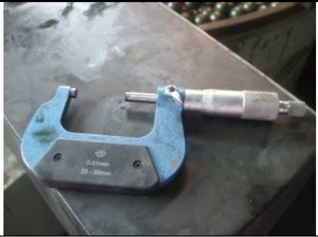
Photo 16 Micrometer without calibration status
