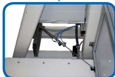
The machine's fully automatic door is opened, closed and locked by pressing a button.
