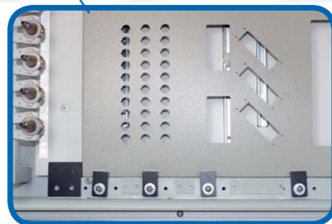
Pneumatic frontside part fixture 7 pneumatic muscles at the base of the machine's frame hold flat workpieces in place at the push of a button. The muscles can be switched off individually to avoid blocking areas in the clamping range. The coating under the fixing points remains undamaged.
