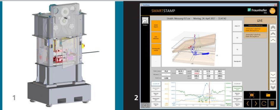
1 Eccentric press with sensors for condition monitoring
