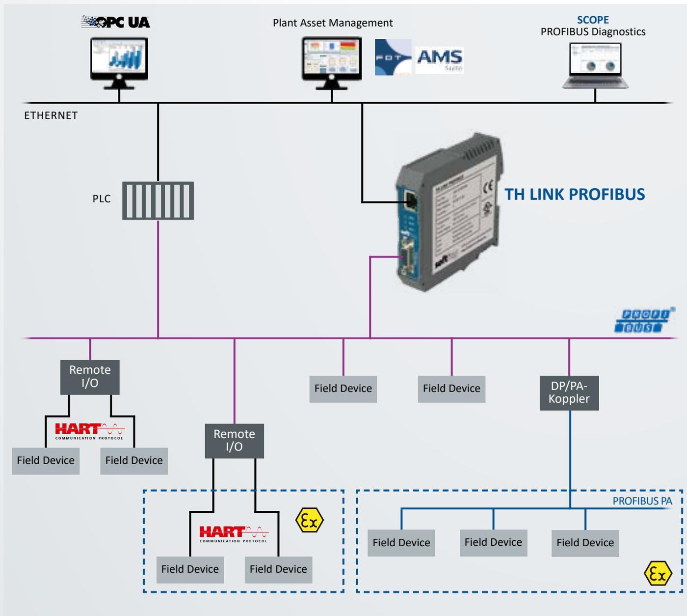
**TH LINK PROFIBUS – PROFIBUS DP network access for Plant Asset Management and Network Monitoring**
