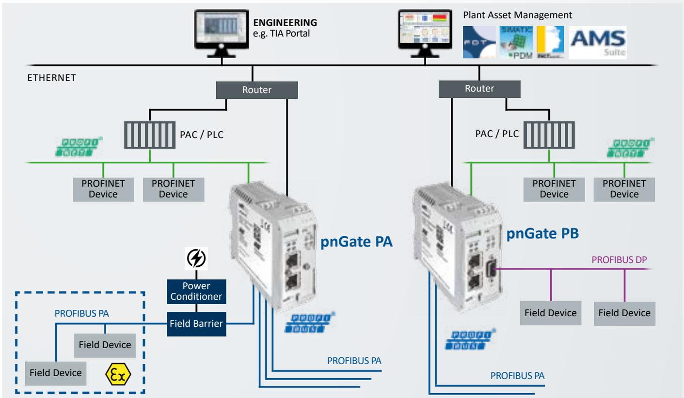
**pnGate PB – Integration of PROFIBUS networks in PROFINET systems**
