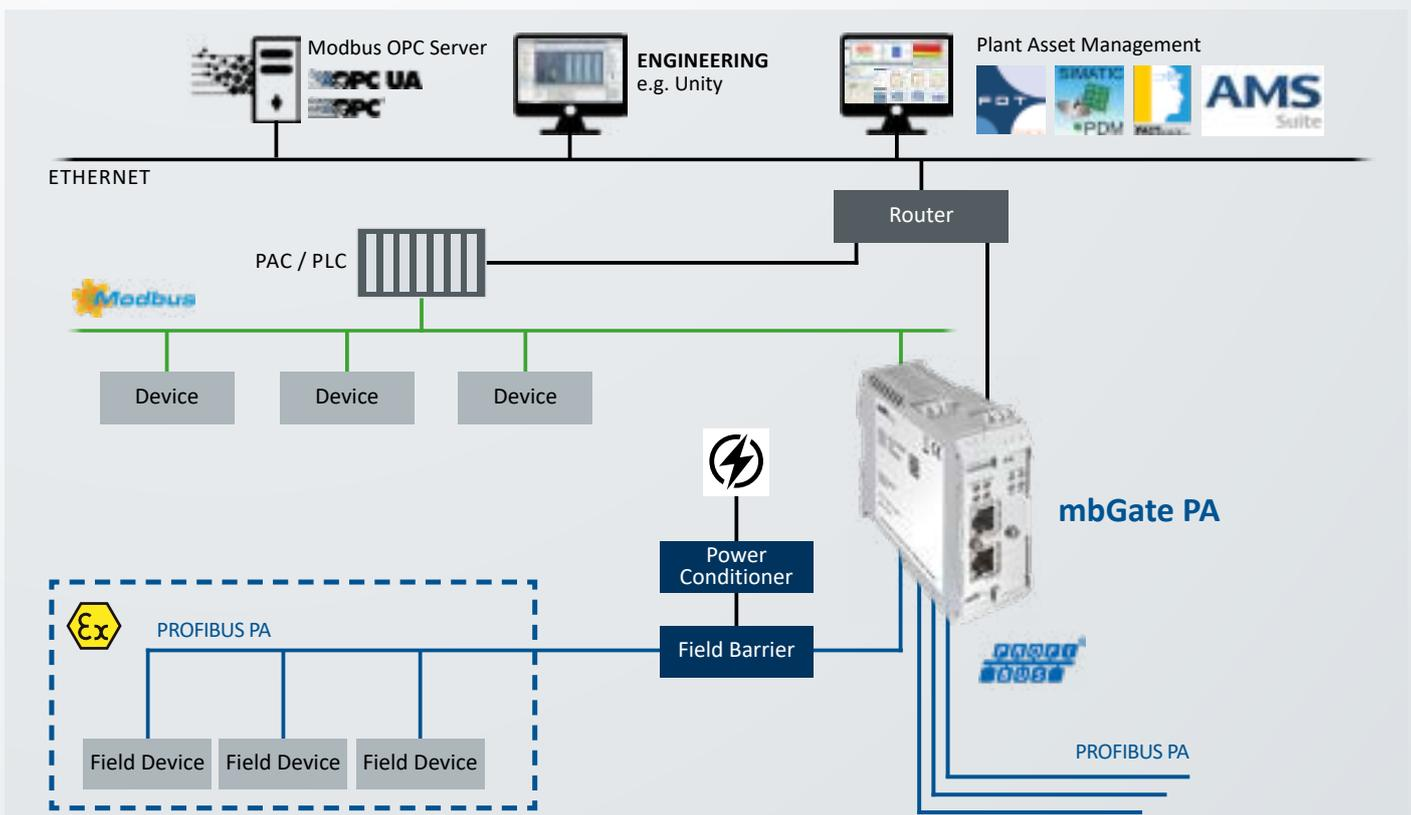
**mbGate PA – Direct integration of PROFIBUS PA segments into Modbus TCP systems**
