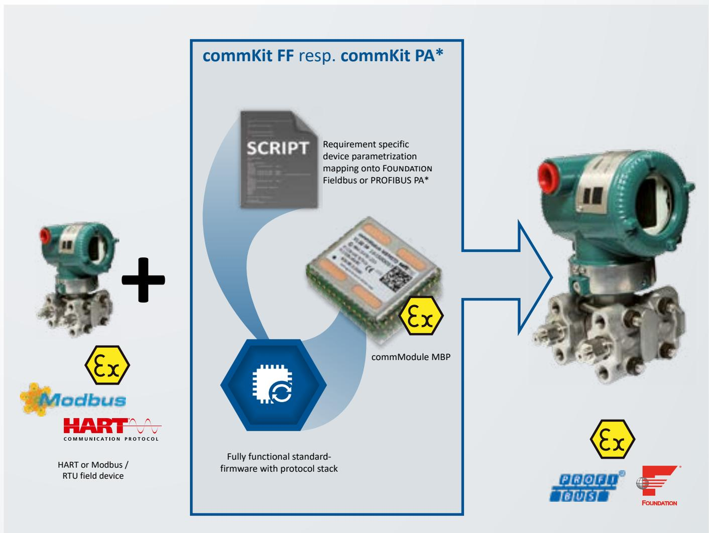
**commModule MBP** – Universal hardware for FOUNDATION Fieldbus and PROFIBUS PA\*
