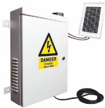
Wireless Electric Measuring RTU is designed for 110–400V AC power distribution system, it can as smart meter to measure current, voltage, power, active power, frequency, etc. If any item exceeds the pre-set value, then it will alert by SMS or voice call, also can be used for monitoring the safety and security of the transformer, e.g. overload, phase loss, oil temperature, oil level, burglarproof, fall down etc. Can cascade various smart meters via RS485.
