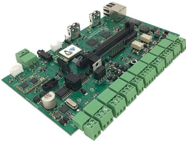
Another example geared more towards home control is the CM3-Home by Guiott (manufactured by Acme systems). The board fits in a DIN-rail enclosure and has a range of useful interfaces and proper 12-24VDC power, but no monitor connector, being a true headless embedded controller. ([https://www.acmesystems.it/catalog\\_cm3home](https://www.acmesystems.it/catalog_cm3home))
