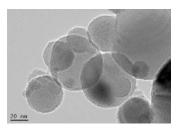
Homogeneous coating on particles
