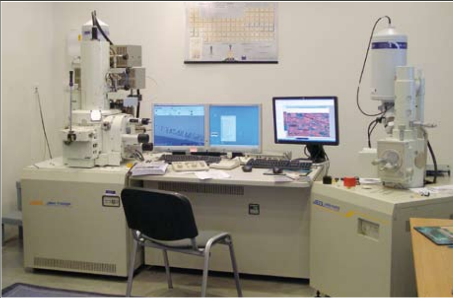
Scanning electron microscopes with EDX analysers and a high-speed EBSD camera
