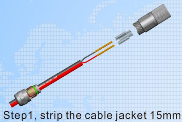
Step1, strip the cable jacket 15mm
