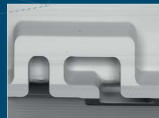
Milled part of a mold. Mill 100 µm
