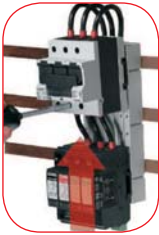
1. Place the component on the top mounting rail and connect 2. Place the component on the lower mounting rail. Position the lower mounting rail to suit component and then connect.
