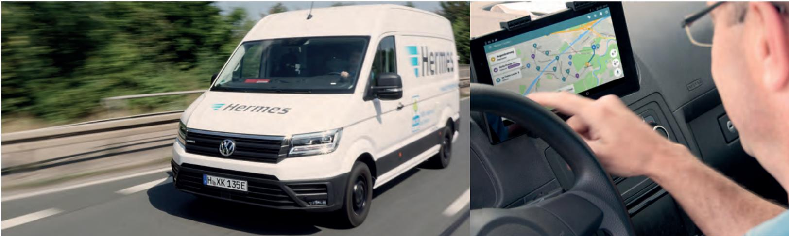
NUNAV Courier transfers all delivery addresses for the current route onto the tablet computer; the driver can follow the recommended route by means of a turn-by-turn navigation.
