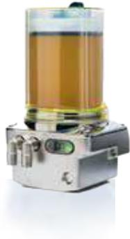
The battery-operated variant of the Lubricus lubrication system is always used when an autarchic operation is desired or necessary. The highly-efficient battery pack can optionally be set to empty the lubricant cartridge over a period of 1–36 months.
