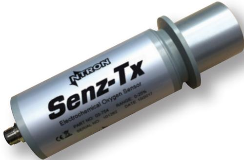
The Senz-Tx is a highly reliable and cost-effective two-wire, loop-powered oxygen transmitter which employs zirconia technology. The Senz-Tx has an analog 4 to 20 mA and RS 485 Modbus communication. It has a measurement range from 1 ppm up to 25% oxygen.
