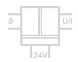
The programmable Temperature Transmitter DT 45000 is used for measure industrial process signals. It converts Pt, Ni, KTY or TC sensor signals as well as poti, resistor and mV signals to isolated standard signals.
