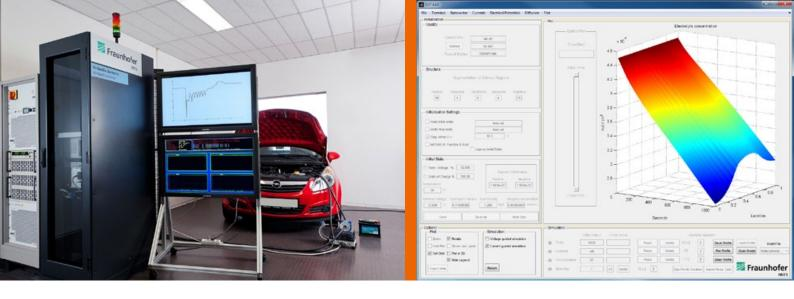
Simulations and "Hardware in the Loop" tests play an important role in modern development processes, since they promise significant time and cost savings. This applies also to the area of electrical systems, where storage devices, such as Lead Acid batteries often are a key component. For such applications Fraunhofer IWES offers a detailed simulation model known as ISET-LAB.
