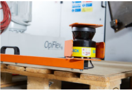
Safety is ensured by two S300 Mini Remote from Sick, which are permanently installed on the mobile robot cell. (Picture: SICK AG)
