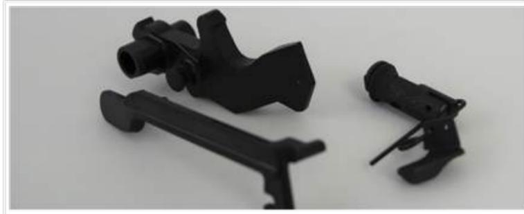
Manganese phosphating (or phosphating) is a dark gray coating of phosphate material with anti-rust and anti-seize properties. The color tone and the thickness of the phosphating depend both on the type of material and the parameters of the bathroom. Manganese phosphating has the advantage, compared to other surface treatments, to guarantee a constant thickness coating over the entire surface.
