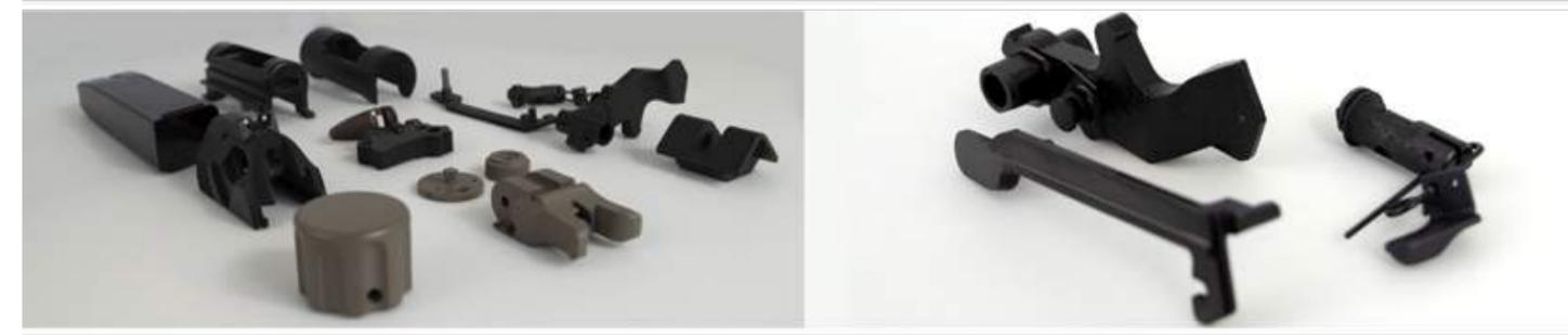
It is an electro-static spray painting based on teflon black color "bruniton type" that is tendentially opaque. Once deposited, it is polymerized at a temperature of 210 ° C in a suitable oven. The parts treated with painting must first be prepared by mechanical sandblasting and manganese phosphating in such a way as to obtain the ideal gripping conditions.
